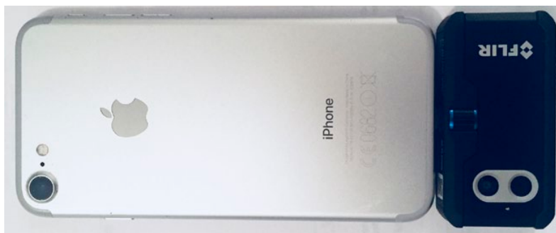
Figure 2. The smartphone (left) and integrated thermal camera (right).
