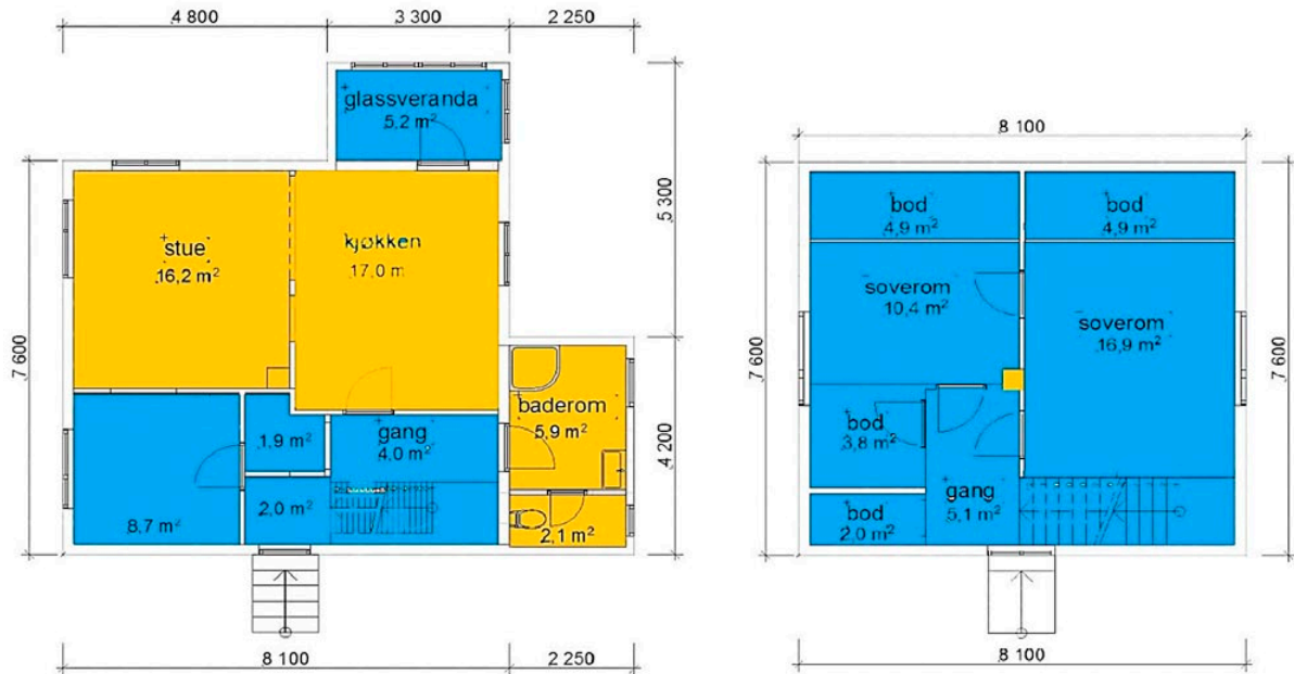
Figure 2. First and second floor in Villa Dammen. Yellow colour shows the area that is permanently heated, including the centred new brick stove. The wall between the two larger rooms in the first floor is removed. The basement is not shown and has not been included in the energy modelling. Second floor rooms are indirectly or intermittently heated.
