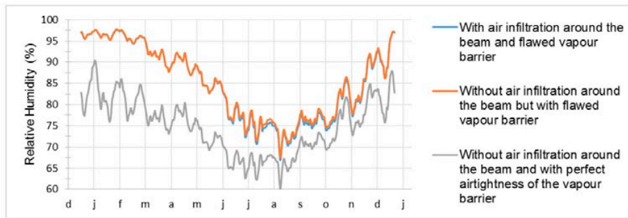
Figure 5. Impact of air infiltration around the beam end and of realistic flaws in airtightness for a configuration with cement lime plaster as external coating and cellulose wadding as insulation material. (Indicator C)
