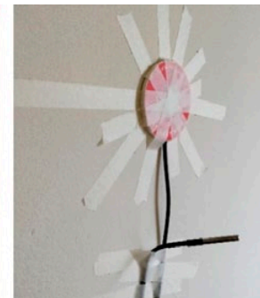
Figure 8. A heat flux meter and temperature sensor integrated in the hybrid-WSN solution.
