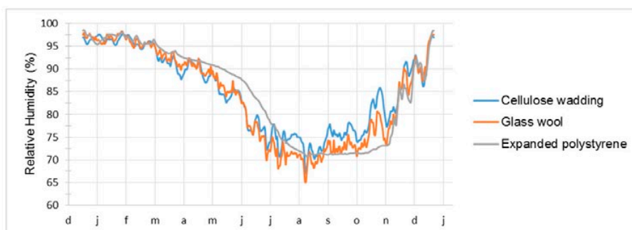
Figure 7. Indicator C with the 3 different insulation scenarios for the configuration with lime plaster as external coating and north façade.
